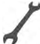
37 Schraubenschlüssel 22-24 mm
